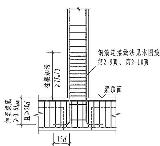
**梁上起柱KZ纵筋构造**
